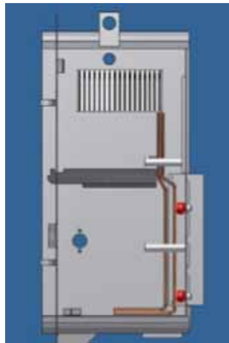
Figure 5- Stand Off Insulators
